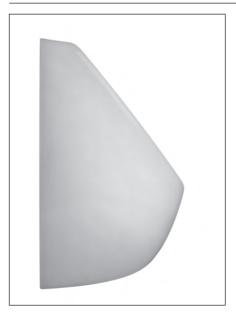
A wall hung urinal of modern design with concealed integral trap and bracketing to provide a smooth easy to clean outer shroud for low cost maintenance. A unique feature of this urinal is the integral air break system for **direct** mains pressure connection. The box rim flush provides for the wash down of the entire inside area of the bowl on each flush. The grate is vitreous china and factory fitted. **Integra** urinal Code No.665102W.
