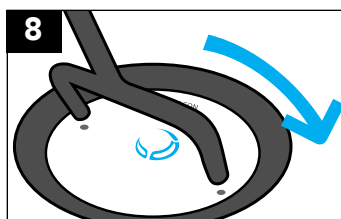
Insert new cartridge into housing and turn key to right (clockwise) to lock and click into place.
