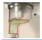
Competitive technology splashes, which causes build-up in housing and pipes.
