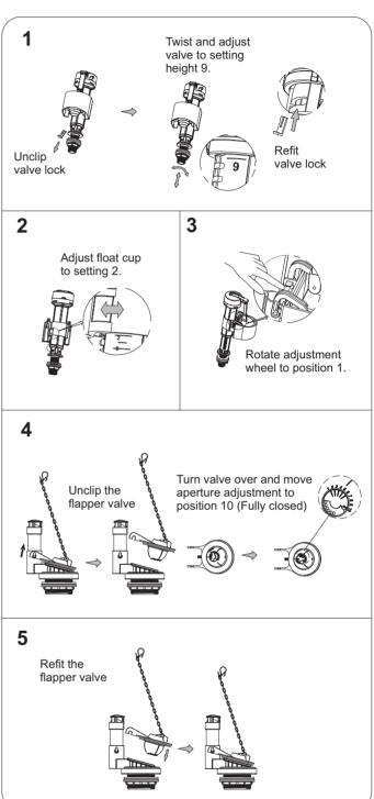
Note: The cistern is supplied with the flush volume set for a single stall installation (1.5L nominal). The valves must be reset as above for a double stall installation
