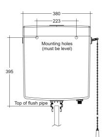
2. Connect the flush pipe to the urinal and the cistern and locate the position of the mounting holes.
