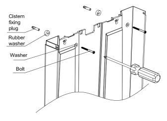
4. Fit the flush pipe to the cistern - assembling the components in the order shown on the diagram.
