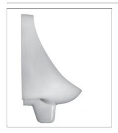
A general application wall hung urinal with integral trap. An adjustable spreader is suitable for installations with increased cistern head height. The spreader channels water to the front and back areas providing a wash down of the bowl on each flush. Available with back inlet and with a stainless steel grate as standard. Concealed cistern and plumbing fittings provide space saving, ease of cleaning and performance matched components to maximise low volume flushing efficiency.
