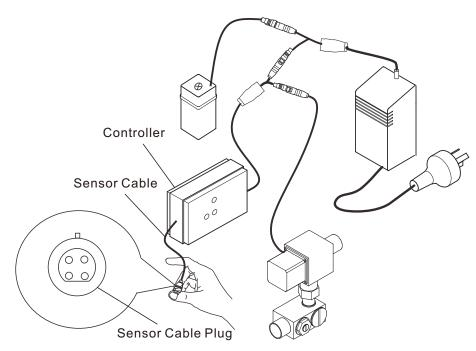
Unplug sensor cable and rub thumb over 4 metal pins. The red light will flash, stop rubbing pins after 20 seconds, the red light will stop flashing, the solenoid will be activated, and the urinal will flush.
