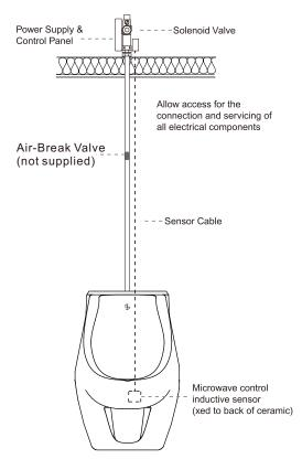
**IMPORTANT**: In-ceiling installation – Installation of air-break valve is recommended. Flush Valve must be installed vertically. Flushpipe must be vertical and straight. Use Copper pipe for flushpipe, DO NOT use flexi hose and ensure no bends/kinks or horizontal pipework. Incorrect installation WILL NOT be covered by your warranty.
