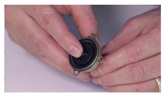
Step 15: If the diaphragm is moving freely, the valve can be reassembled by reversing the steps above.
