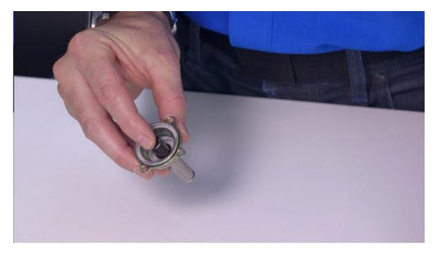
Step 14: Place the diaphragm back on top of the shaft and make sure it moves freely up and down when pressed together.
