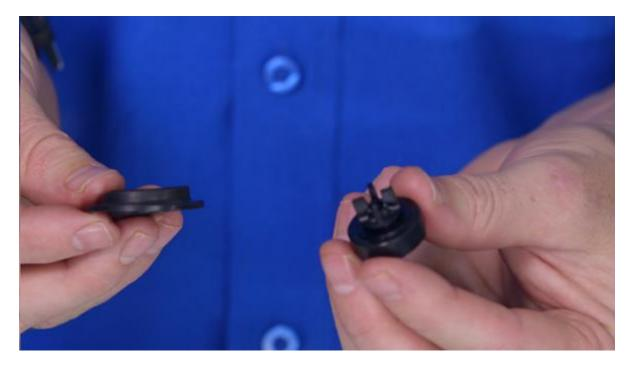
Step 10: Check the shaft of the valve by holding it upside down and tipping out the components into your hand. See if there is any grit or foreign objects within the shaft.
