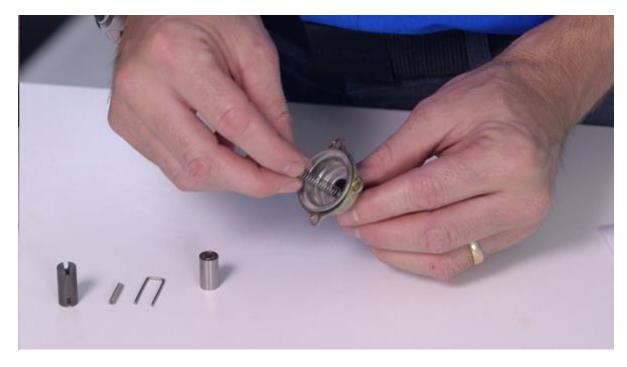
Step 12: Place the bullet into the shaft spring then insert the small spring into the second bullet which has a seating rubber in the top which sits against the diaphragm.
