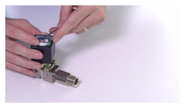
Step 4: Then remove the white washer, the wingdings and the wave washer.
