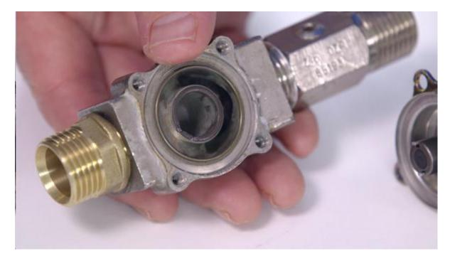
**Step 9: Check** the **diaphragm for wear, cuts, nicks or holes.** If you find evidence of wear, or if you see any black marks on your fingers, you will need to replace the diaphragm with component 90279. Please contact Zip Customer Service on 1800 42 43 44 to order a replacement part.
