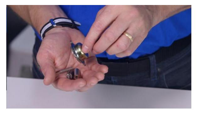
Step 11: Wash the parts then reassemble them. Put the shaft between your fingers and insert the large spring – it goes into the bullet that has an insert for the spring.
