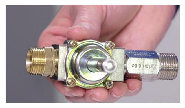
**Step 6:** Carefully **undo the screws**, taking care to hold down the valve top as the fourth screw is removed so the two springs and two bullets inside the valve do not shoot out.
