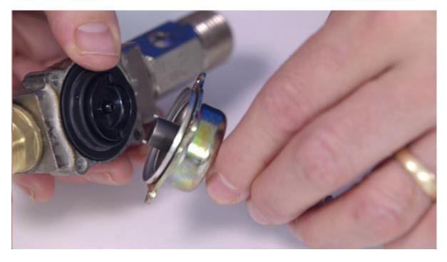
**Step 8: Check** the seat of the **valve for wear or damage**. If you see evidence of wear you will need to replace the valve body with component 90590 or the complete valve. Please contact Zip Customer Service on 1800 42 43 44 to order replacement parts.
