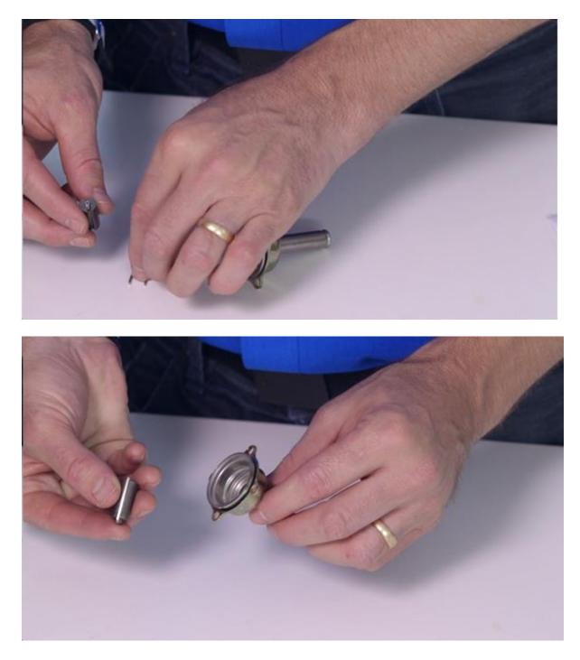
Step 13: Insert the u-bracket wire into the shaft spring and u-bracket.
